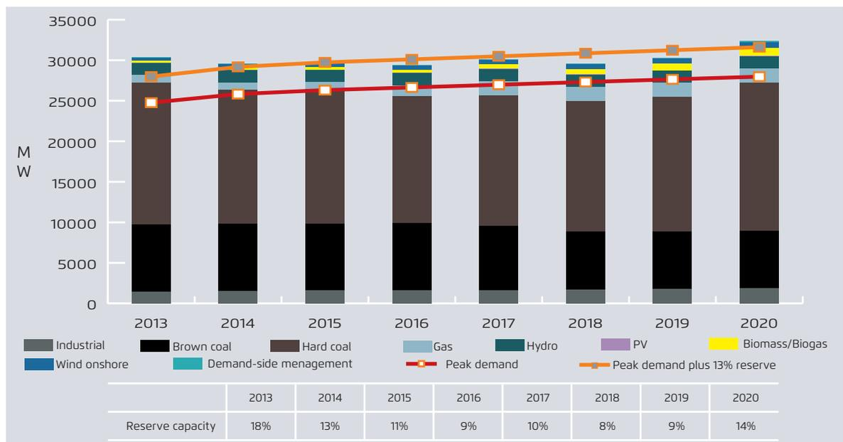
**Fig. 1b. Power balance on the National Electricity system up to 2020, taking into account the cold reserve.**
